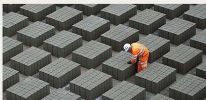
Lightweight concrete blocks with recycled content including fly ash and crushed demolition waste.
