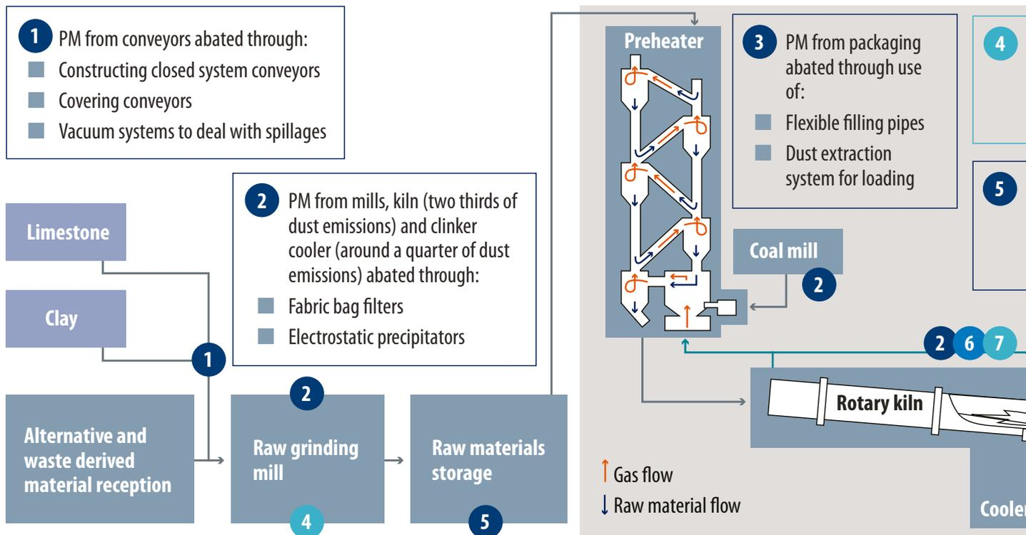
Figure 7: The cement manufacturing process and the emission of NO<sub>x</sub>, PM and SO<sub>2</sub> and their abatement
