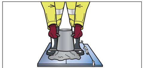
Figure B.8 Lift the cone carefully
