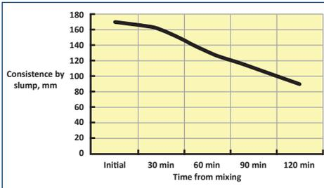
Figure 1 Example of slump loss with time
