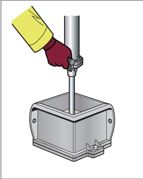
*Fig D.6 Compact 50 mm layers with vibrating hammer*
