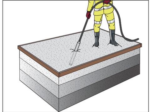
**Figure 8. Compaction by internal vibrator, or poker.**
