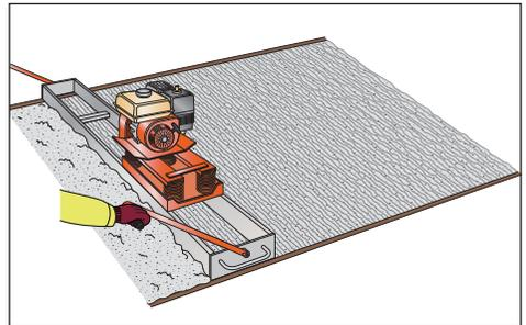
**Figure 11. Slab compaction using a vibrating beam**
