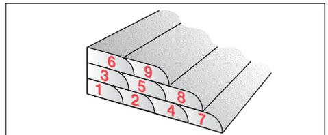
**Figure 7. Placing sequence to avoid cold joints.**
