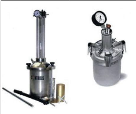
*Fig C.1 Water column test apparatus*
