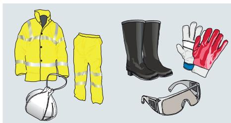
**Personal Protective Equipment (PPE) for working with concrete.**
