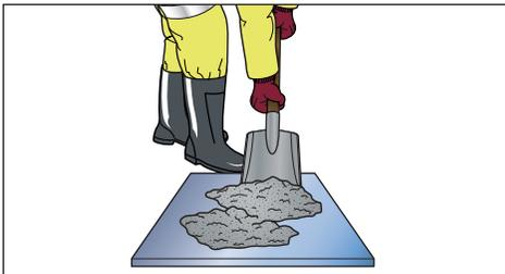
Figure B.1 Remixing sample on tray
