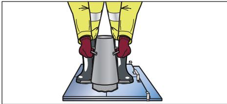
Figure B.4 Lifting Cone
