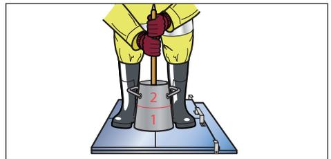
Figure B.7 Filling cone and tamping
