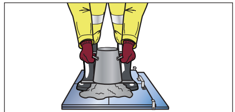
Figure B.8 Lift the mould carefully
