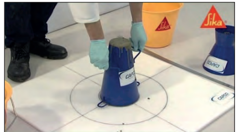
Figure B.11 Slump-flow cone ready for lifting
