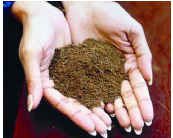
The cement industry uses far more waste than it produces – such as this sterilised meat and bone meal for kiln fuel
